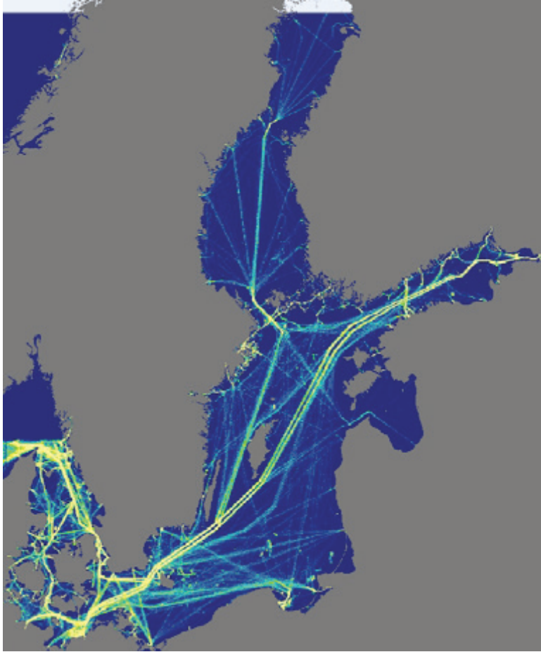
Figure 1. The density of ship traffic during one week in 2008, with the busiest routes in the Baltic highlighted in yellow (HELCOM, 2009). Note the clearly visible traffic separation lanes (e.g., north-south bound) which is an example of an Associated Protection Measure (APM) of the Baltic's Particularly Sensitive Sea Area (PSSA) designation.
